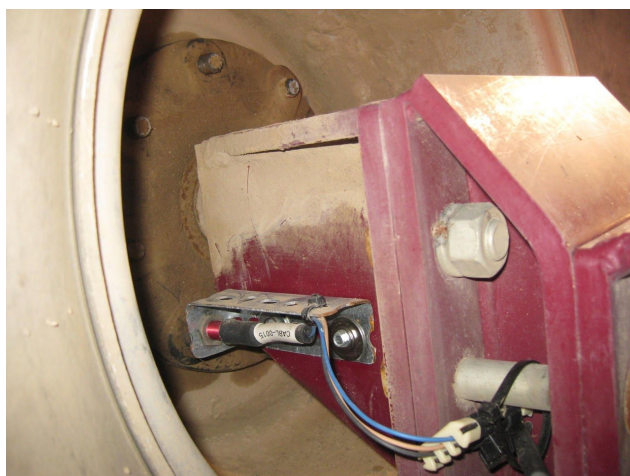
Figure 8: Wheel Sensor installed on a sprayer, Axle and Wheel shown also. Install with around a 1/16 inch gap between sensor and lug bolts.
