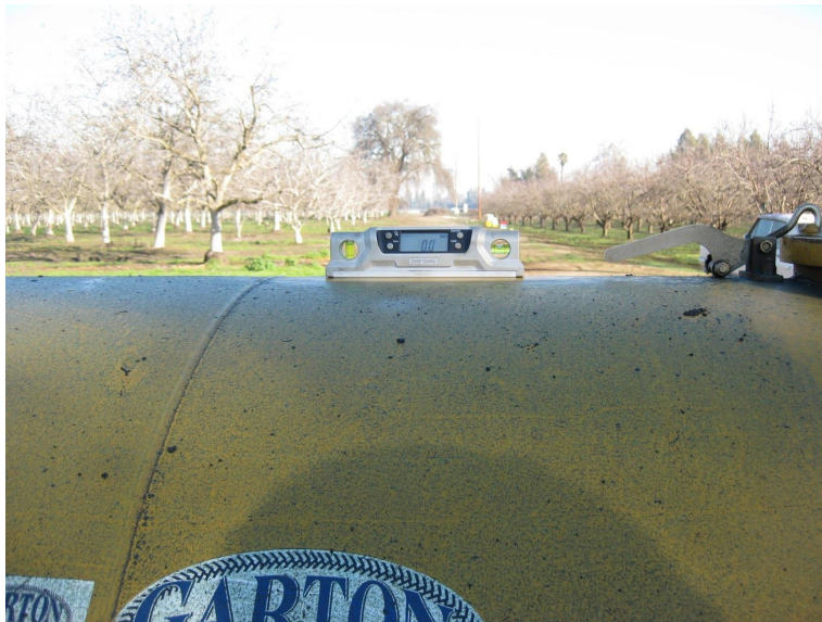
Figure 27: Level on Orchard Sprayer verifying it is level before starting calibration
