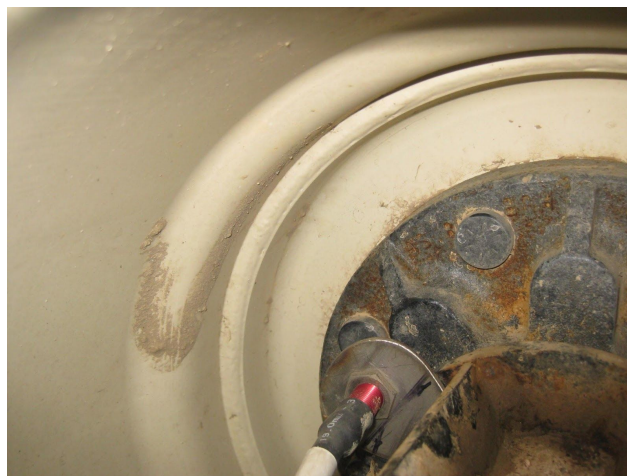
Figure 8: Wheel Sensor installed on a sprayer, Axle and Wheel shown also. Install with around a 1/16 inch gap between sensor and lug bolts.
